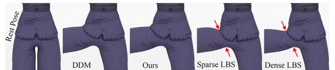
Fig. 7. Utilizing “negative bulging” effect, DDM (variant 0) and our model can resolve the collapsing issue near the hip joint. Dense LBS, which is DDM variant 5, shows less artifacts than Sparse LBS, which is the original data from Mixamo. Our method is shown on Ninja 500 test data.
